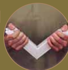
Pinch fusion welding
